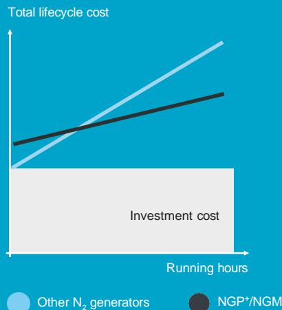
With an air factor\* of 1.8 (at 95%) to 5.5 (at 99.999%) and a special cycle time modulation algorithm, the running cost of the new NGP<sup>+</sup> can be reduced by 50%, compared to other N<sub>2</sub> generators.
